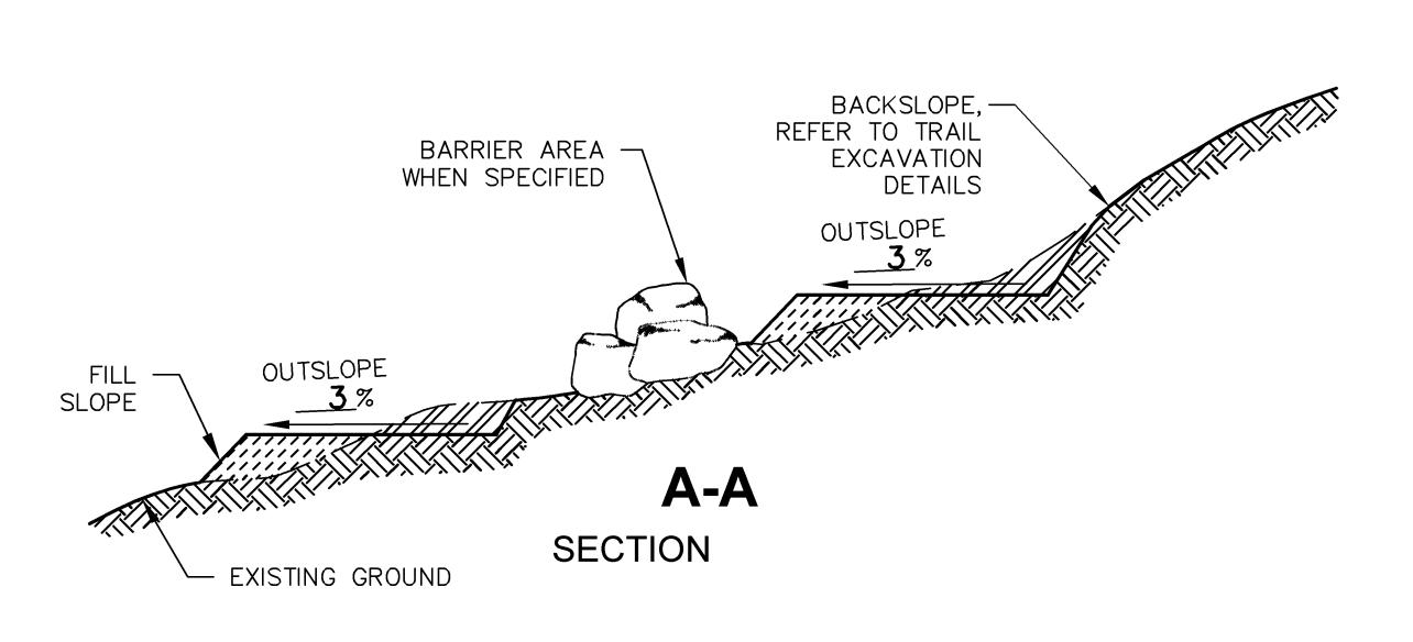
CONSTRUCT CONSTANT GRADE THROUGH BOTH APPROACH SECTIONS.
